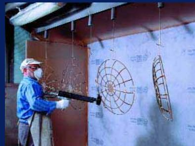
This is where protective lacquer is applied, giving a durable and resilient quality to the products' surfaces. Most of the parts are lacquered by hand in an electrostatic process and then fired in a hardening kiln at 120° C. Once the drying process is complete, employees check all the parts once again before preparing them for installation.
